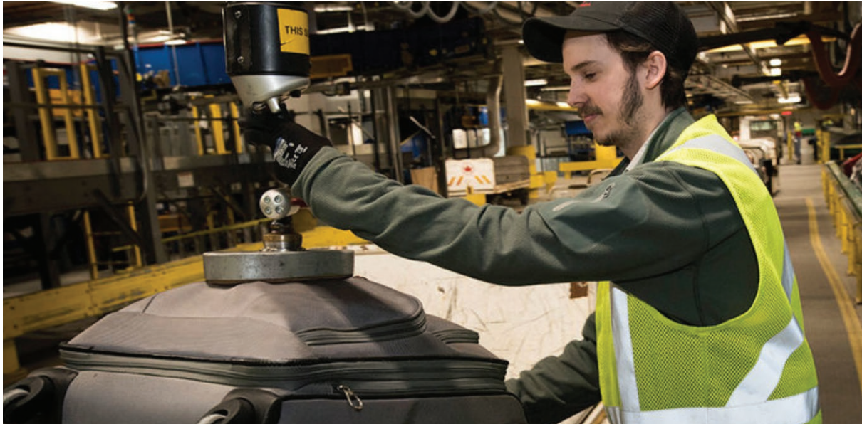
Jack Normand, Air Canada baggage handler, uses the Vacu-Lift to safely move bags from the carousel to the loading carts. The Vacu-Lift can help employees like Jack safely handle hard and soft-sided luggage weighing up to 150 pounds.
